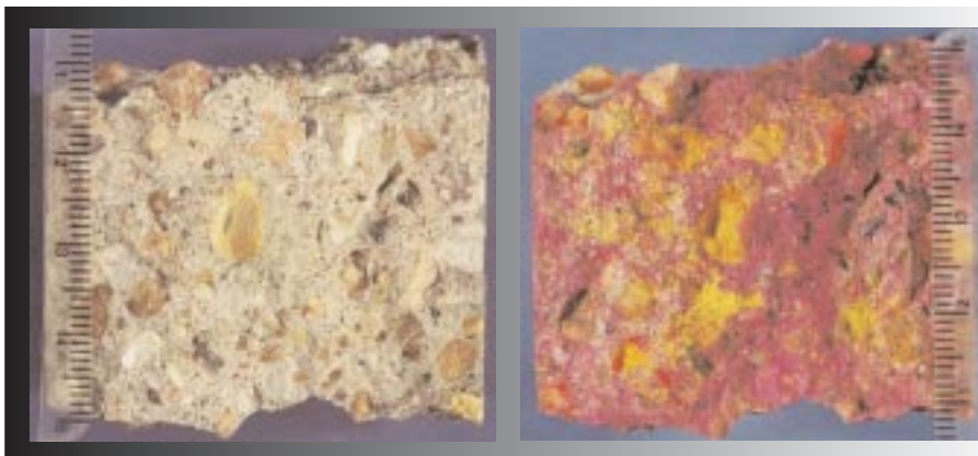
Fig. 3. Concrete as it appears before (left, #68939) and after (right, #68940) staining with solutions from the Los Alamos Method.
