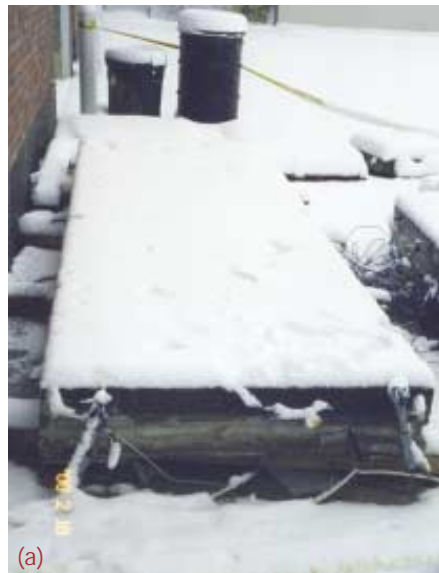
Fig. 5: The 1.2 x 3.6 m (4 x 12 ft) slab during experiments in the winter of 1999: (a) slab before testing; and (b) slab during testing
