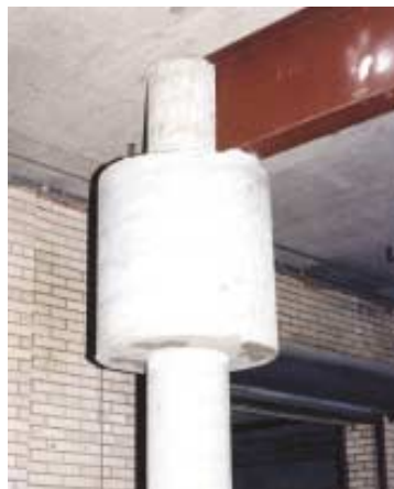
Fig. 10: Eccentrically loaded shear collar
