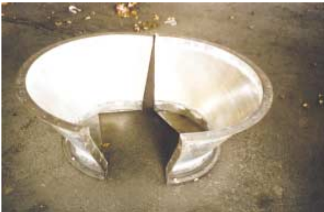
Fig. 5: Reusable steel form for sloping column surface
