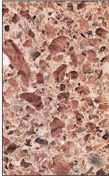
Abrasive blasting fractures the surface of aggregate particles and tends to mute their color. Compare aggregate exposure by retardation (left) with the sandblasted finish on the right. These are actual size samples of identical concrete, made with 1/2 x 3/4-inch ruby feldspar coarse aggregate, white cement, and ruby feldspar sand.
