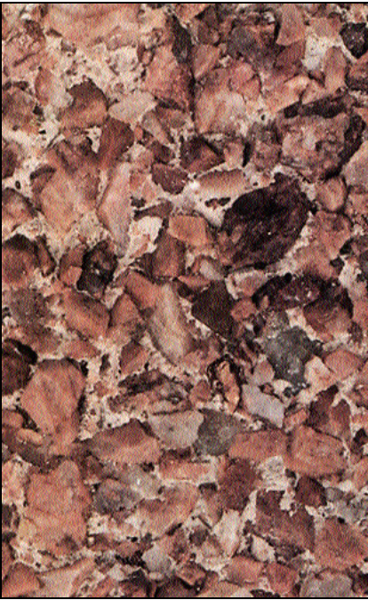
Abrasive blasting fractures the surface of aggregate particles and tends to mute their color. Compare aggregate exposure by retardation (left) with the sandblasted finish on the right. These are actual size samples of identical concrete, made with 1/2 x 3/4-inch ruby feldspar coarse aggregate, white cement, and ruby feldspar sand.
